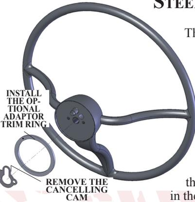
The spline in your stock steering wheel is the same as the one on the new column, so no modifications are needed here.
