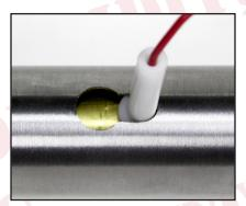
12. Connect the horn plunger wire to the negative side of the horn relay or simply follow the directions in your wiring kit.
