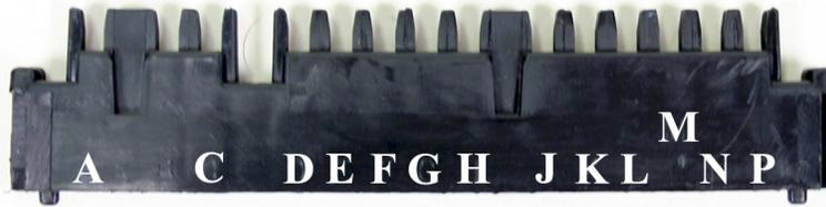
The female side to the male plug on our column has been provided with the column. There are eight crimp-on clips that will need to be attached to the following wires on your vehicle, then plugged into the corresponding position in the harness. The female plug is not the exact length of the male plug, however, they will connect properly.
