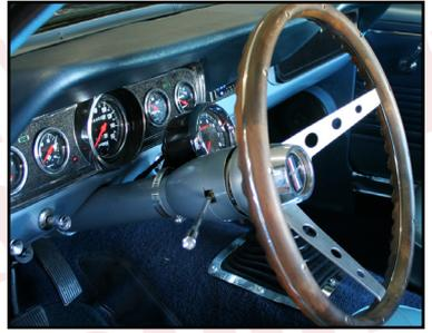
Remove the nut and use a wheel puller to pull the original steering wheel off the original column. (Figure 1)
