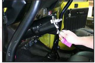
Turn two clicks forward. This should turn the accessories on and the ignition system on. (coil or electronic ignition has power)
