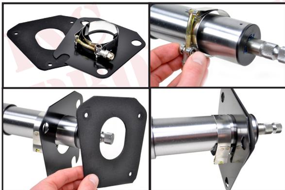
**Note:** When you install your new floor mount you will notice that the column tube at the upper end is 2 1/4" while the lower part of the tube is 2" in diameter. The column is made to collapse as was the original, only in a different way.
