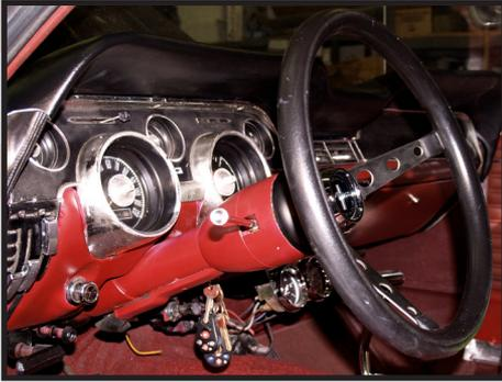
Remove the nut and use a wheel puller to pull the original steering wheel off the original column. (Figure 2)
