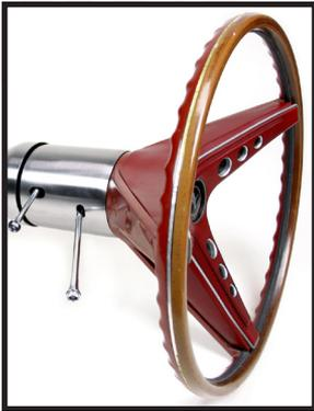
**OEM Wheel - Must be for the same year application as the column. *\*Use of a different year of wheel will result in damage to the turn signal switch.\****
