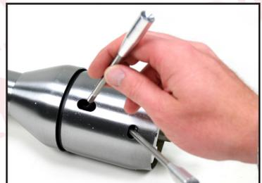
The turn signal lever (longer of the two levers) is installed into the threaded hole closest to the top of the column.
