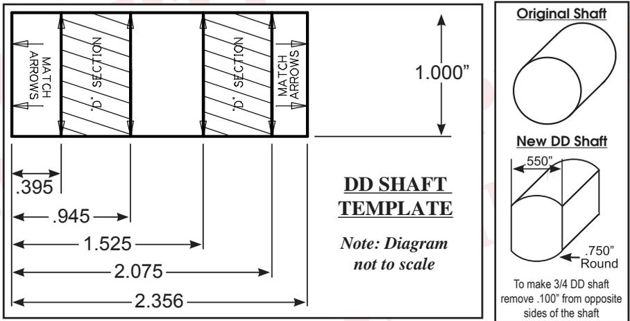
Starting from an 1/8 from the bottom, wrap the paper template around the shaft and match the horizontal arrows together.
