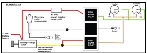
**Diagram 1B.** Installation of the switching module on a typical dual headlight system using a separate 12 volt power source for the high beam relay. This is the same situation as described in Diagram 1A. If you have an available 12 volt power circuit, this connection can be used. A separate circuit breaker is still required to protect the high beam relay power input circuit.
