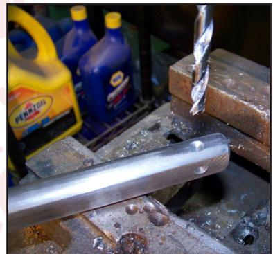
use a 1/4 inch drill bit and create a relief for the setscrew. This relief only needs to be approximately 3/16 inch deep.
